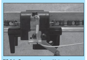
FIG. 6-4 Emergency release cable to carriage.
